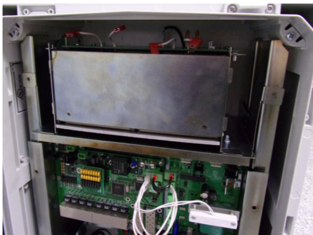
Figure 7.1 – Battery compartment removal
